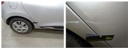
Wheel cover R L, Crack, E - Replace
