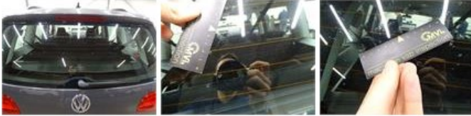
Roof pillar L, Dent(s), Acceptable
