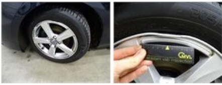
Alloy rim F L, Deformed / Strained, E - Replace
