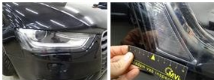
Headlight sprinkler cover R, Broken, E - Replace
