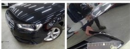
Xenon headlight L, Scratch(es), 67 - Polish
