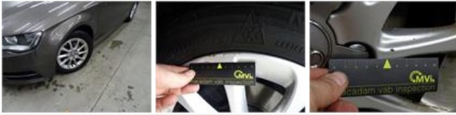
Alloy rim R L, Scratch(es), Acceptable
