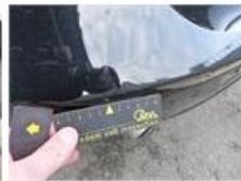
Bumper R, Dent(s) and scratch(es), LI - Repair and paint (complete)
