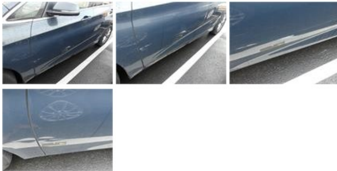
Door R R, Dent(s) and scratch(es), Le - Replace and paint
