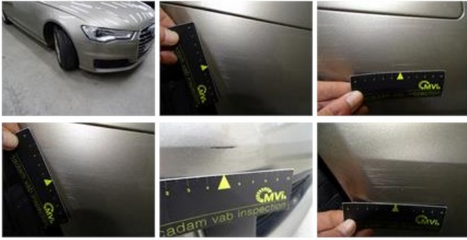
Bumper F L, Scratch(es), It - Spot repair
