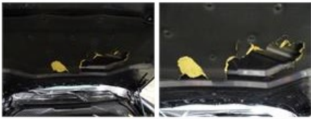
Backrest cover F L, Damaged, Acceptable
