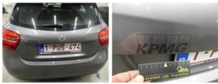
Bumper R, Dent(s), LI - Repair and paint (complete)
