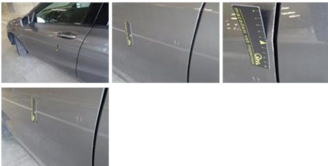
Door R L, Scratch(es), LI - Repair and paint (complete)
