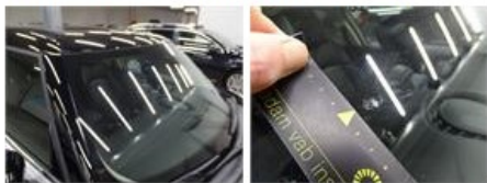
Tailgate, Chemical polution, Acceptable
