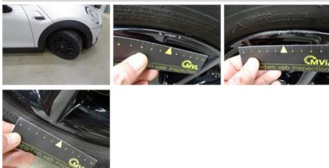
Door R L, Dent(s), PDR - Paintless dent repair
