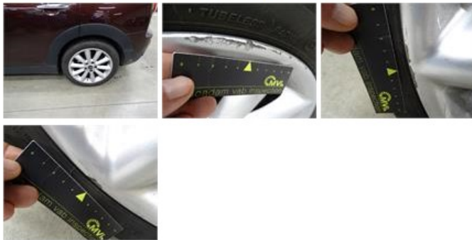
Door F R, Scratch(es), LI - Repair and paint (complete)
