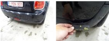
Sill trim L, Broken, E - Replace
