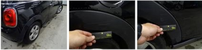
Door F L, Dent(s) and scratch(es), LI - Repair and paint (complete)
