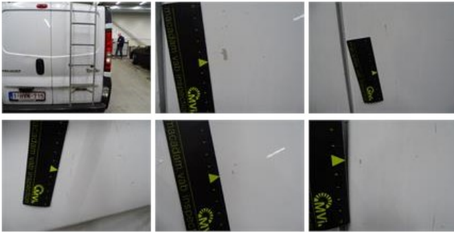
Central pillar L, Dent(s) and scratch(es), LI - Repair and paint (complete)
