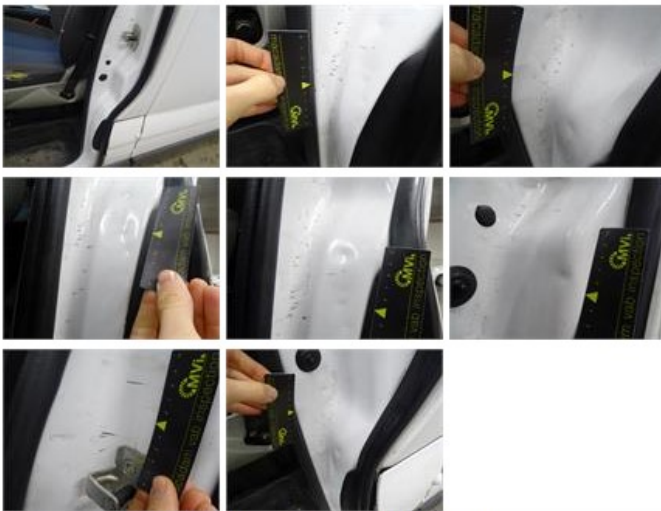
Roof, Deformed / Strained, LI - Repair and paint (complete)
