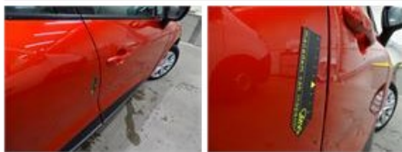
Window F L door, Scratch(es), E - Replace
