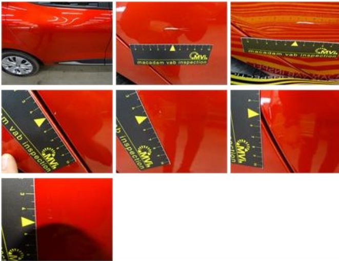
Door R L, Scratch(es), LI - Repair and paint (complete)
