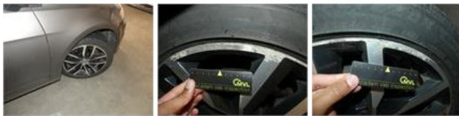
Alloy rim R R polished, Rust, LI - Repair and paint (complete)
