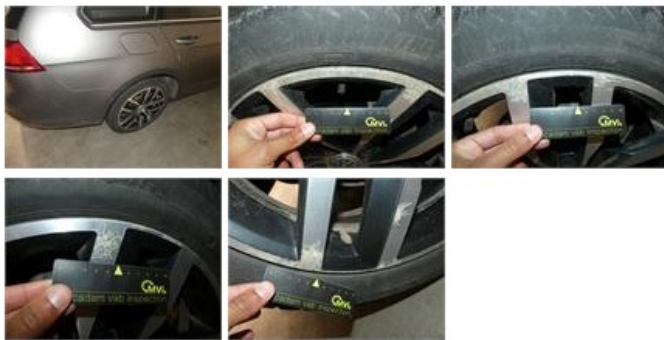
Alloy rim F L polished, Rust, LI - Repair and paint (complete)
