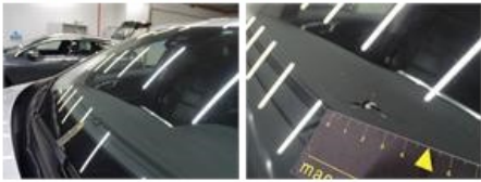
Wing F L, Dent(s), LI - Repair and paint (complete)
