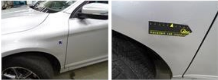
Wing F R, Bad repair, LI - Repair and paint (complete)
