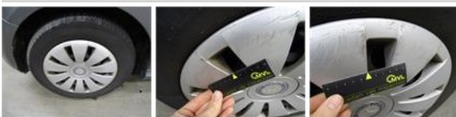
Wheel cover R R, Scratch(es), E - Replace
