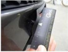
Wheel cover F R, Broken, E - Replace
