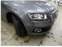
Bumper F, Dent(s) and scratch(es), LI - Repair and paint (complete)
