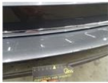
Bumper F, Dent(s) and scratch(es), LI - Repair and paint (complete)
