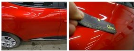
Window R L door, Scratch(es), Acceptable
