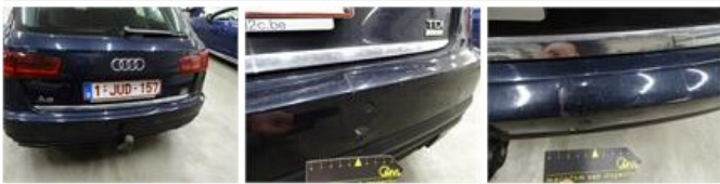
Sill outer R, Scratch(es), LI - Repair and paint (complete)
