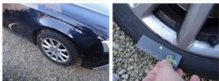
Sill outer L, Dent(s) and scratch(es), LI - Repair and paint (complete)
