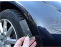
Wing F L, Scratch(es), LI - Repair and paint (complete)
