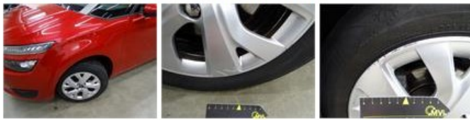
Wing R R, Scratch(es), LI - Repair and paint (complete)
