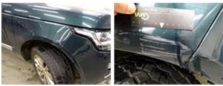
Bumper R, Broken, Le - Replace and paint
