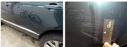
Door F R, Dent(s) and scratch(es), LI - Repair and paint (complete)
