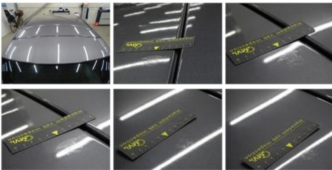
Roof, Chemical polution, 67 - Polish 0,00
