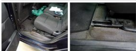
Protection plate M, Tear, E - Replace
