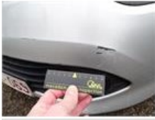
Wing F L, Deformed / Strained, Le - Replace and paint
