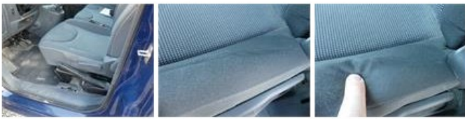
Seat cover F R, Damaged, Acceptable
