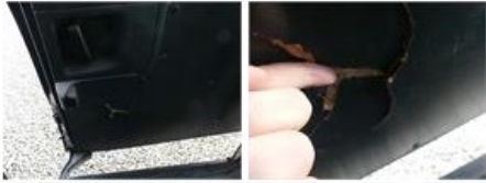
Trunk lid covering R, Hole, E - Replace
