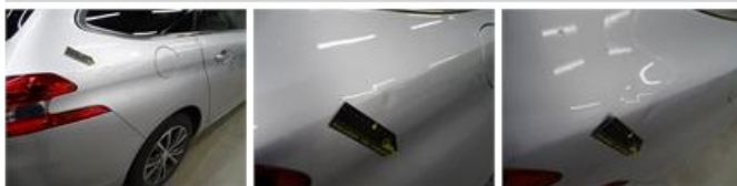
Sill outer R, Dent(s), LI - Repair and paint (complete)
