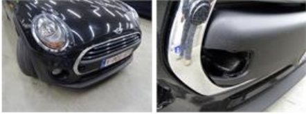
Wing R R, Repaired, Acceptable
