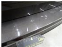
Bonnet, Bad repair, LI - Repair and paint (complete)
