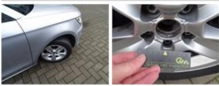
Wheel cover R R, Missing, E - Replace
