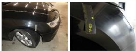
Bumper F, Broken, Le - Replace and paint
