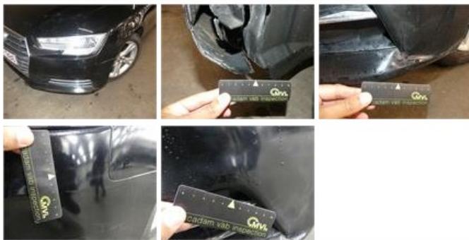
Door F R, Dent(s), LI - Repair and paint (complete)
