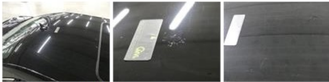
Wing F R, Bad repair, LI - Repair and paint (complete)
