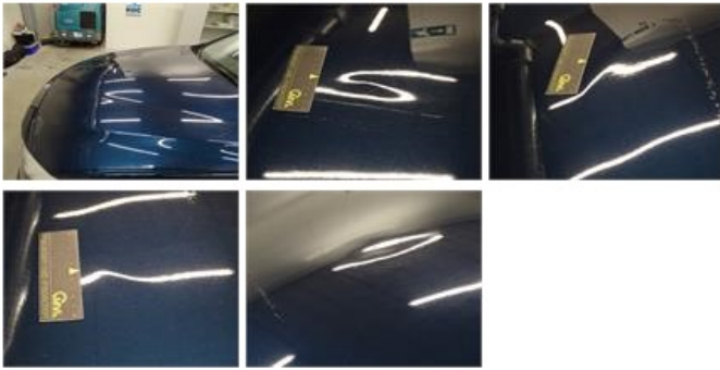
Roof, Dent(s), LI - Repair and paint (complete)
