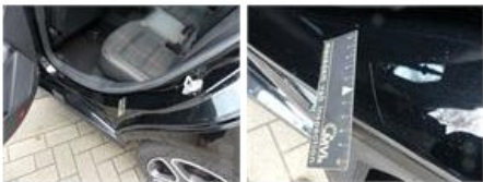
Floor covering F L, Burned, Smart repair
