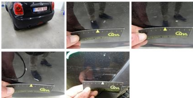
Wing R R, Bad repair, Acceptable
