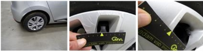
Wheel cover R L, Scratch(es), E - Replace
