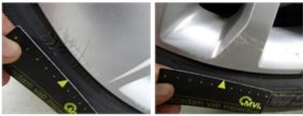
Wheel cover R L, Scratch(es), E - Replace
