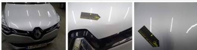
Bonnet, Dent(s), LI - Repair and paint (complete)
