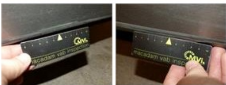
Floor covering F L, Stain, Acceptable
