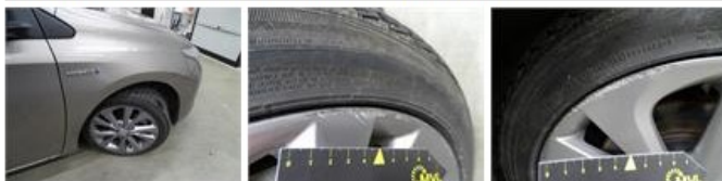
Alloy rim R R, Scratch(es), LI - Repair and paint (complete)
