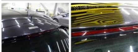
Bumper corner R R, Deformed / Strained, Smart repair
