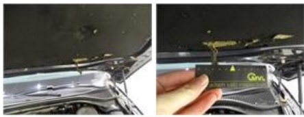
Wing F R, Dent(s), PDR - Paintless dent repair
