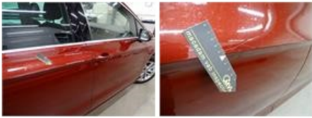
Door frame R L, Deformed / Strained, Repair/replace (lump sum)
