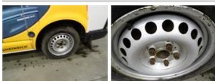
Wheel cover F L, Missing, E - Replace
