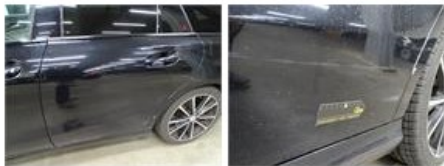
Door F R, Scratch(es), LI - Repair and paint (complete)
