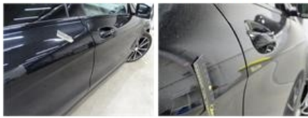
Sill outer L, Scratch(es), It - Spot repair
