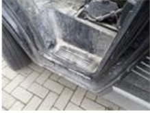
Rocker panel inner F L, Dent(s), LI - Repair and paint (complete)
