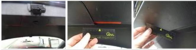
Roof, Dent(s) and scratch(es), LI - Repair and paint (complete)
