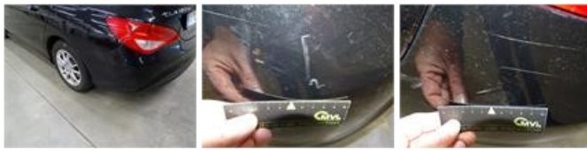
Sill outer R, Scratch(es), It - Spot repair
